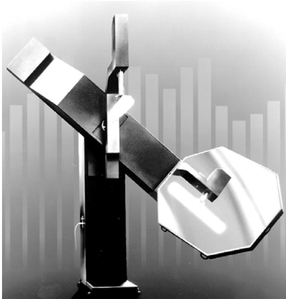
FIG. 1 Rotating mirror goniophotometer (image courtesy LightLab International)
