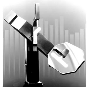
FIG. 1 Rotating mirror goniophotometer (image courtesy LightLab International)
